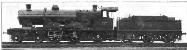
Fig. 5054. Ten-Wheel, Four-Coupled, De Glehn, Four-Cylinder Balanced Compound Locomotive. Great Western Railway. Cylinders 14 13-16 in. and 23 \frac{3}{4} in. x 25 3-16 in.; Working Steam Pressure 227 lbs. per sq. in.; Total Heating Surface 2,755.7 sq. ft.; Weight on Drivers 75,040 lbs.; Total Weight 150,940 lbs.
